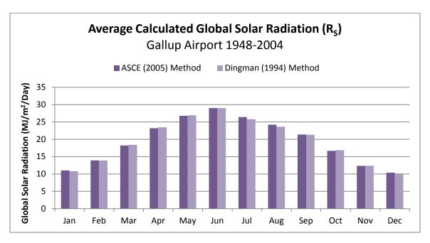
Figure 18 – Comparison of Global Solar Radiation at Gallup Airport (1948-2004) Calculated with Dingman (1994) and ASCE (2005) Equations, filled from Albuquerque Int'l as described in section 2.5.1
