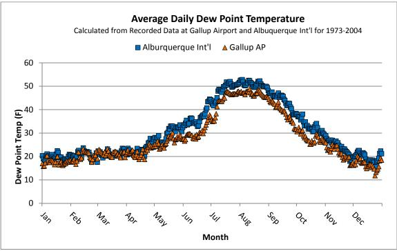
Figure 1 – Average Daily Dew Point Temperature  $(T_{\text{dew}})$  at Gallup and Albuquerque
