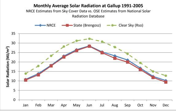
Figure 8 - Monthly Solar Radiation at Gallup, Estimates from NRCE's Sky Cover Data vs. Brengosz (2010)'s Radiation Estimates from NSRDB
