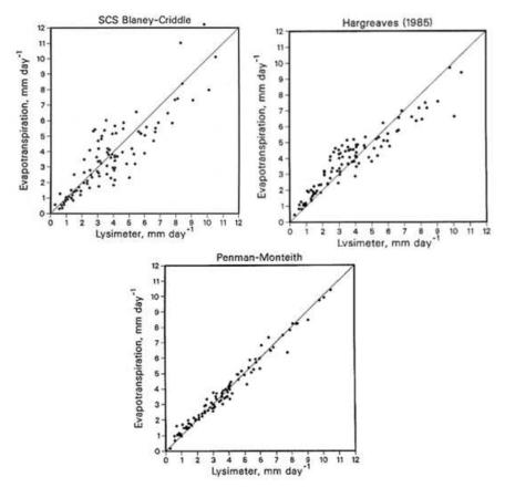
Figure 15 - Estimated ET verses Measured ET (lysimeter) for Blaney-Criddle, Hargreaves, and Penman-Monteith Methods at 11 Locations (Jensen, et al., 1990)
